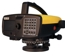
SANDING SL03 32x Magnification Telescope 0.3mm accuracy Invar Staff
